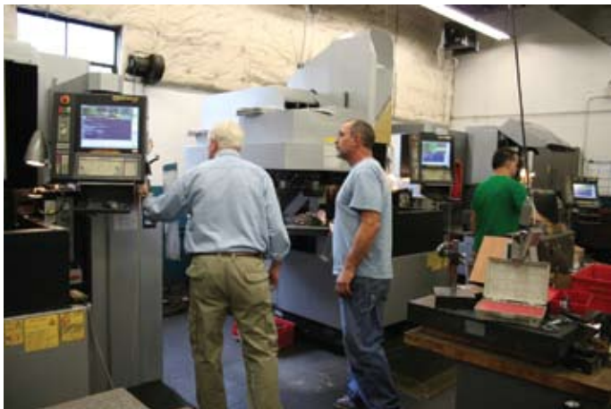
Two brand new Sodick EDMs helped LSR Engineering add LSR molding (liquid silicone rubber/ LIM (liquid injection molding) capabilities to create flashless, automatic running molds for liquid silicone.
