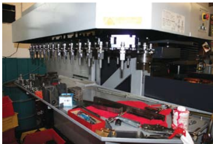
This 32-position toolchanger allows long, uninterrupted EDM operation.
