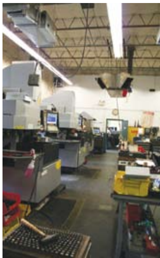
Two Sodick Ram EDMs and one Sodick Wire EDM are amongst the more than $1 million LSR Engineering has invested in equipment upgrades.
